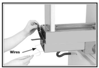
Figure 50. Neoprene shipping seat wires.
